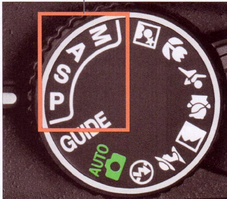
Figure 7-8: You can control exposure and certain other picture properties fully only in P, S, A, or M mode.
